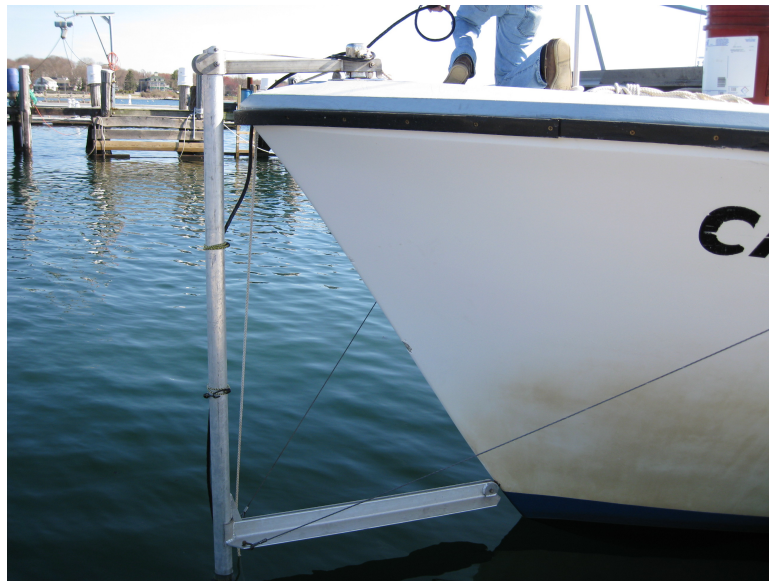
Fig. 5. Aluminum bow mount on the Cap'n Bert.
